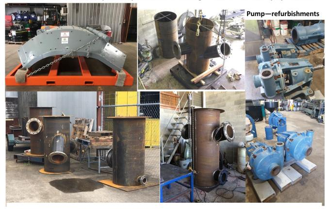
WEAR LINING - Sheet rubber—moulded rubber modules - Moulded Rubber backed Ceramic liners with CN Back— Arco plate—CCO—Polyurethane—Ceramic tiles— Alumina , Zirconia Toughened Alumina, Reaction Bonded Silica Carbied
